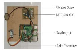
Fig -2: Transmitter Side
