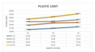
Fig -4: Plastic Limit values for different mix proportions
