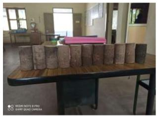
Fig -3: Unconfined Compressive Strength Test Samples
