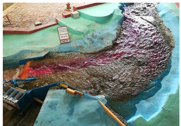
Fig -9: Flow pattern for RDC for 100 year flood (Hydro Lab Pvt. Ltd., 2018)
