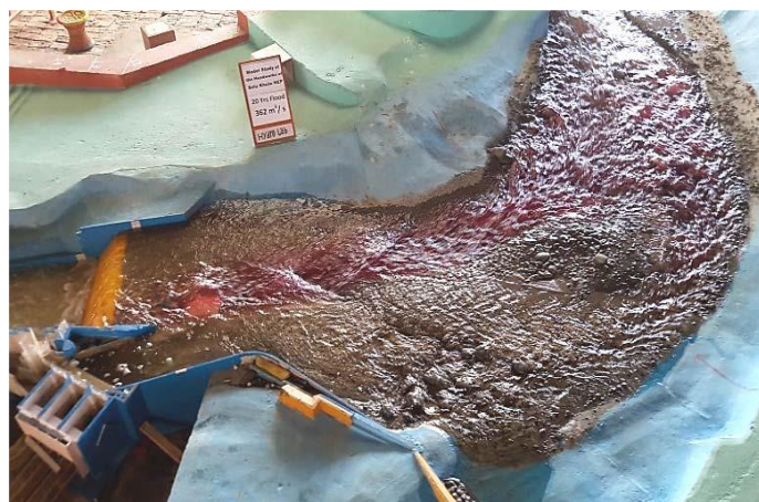
Fig -7: Flow pattern for RDC for 20 year flood (Hydro Lab Pvt. Ltd., 2018)
