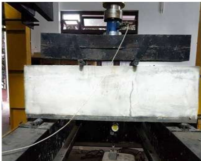
Fig -5: Retrofitted beam
