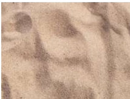
Fig. 3: Sand passing through 600µm sieve
