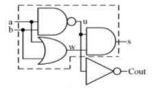
Fig. 2. (a) An accurate half adder
