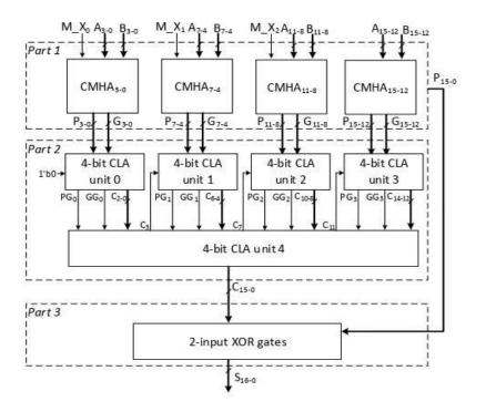
Fig. 1. Structure of the proposed 16-bit adder.
