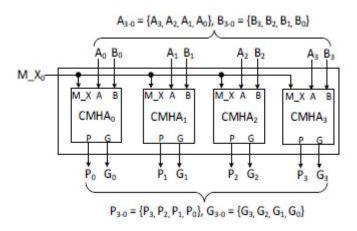
Fig. 4. Structure of a group with four CMHAs
