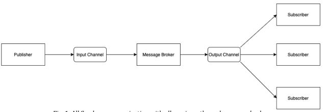
Fig. 1: All Senders communicating with all receivers through message broker
