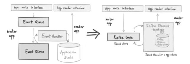
Fig. 4: A basic flow of an event-driven architecture
