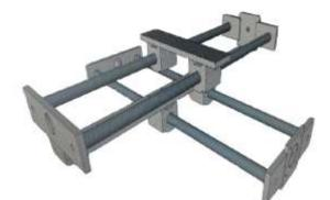
Fig. 3: Design of Cross-Slide
