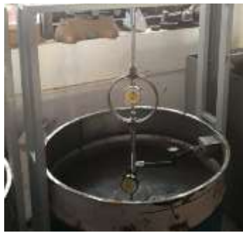
Fig-5 : Experimental setup for initial pile load test
