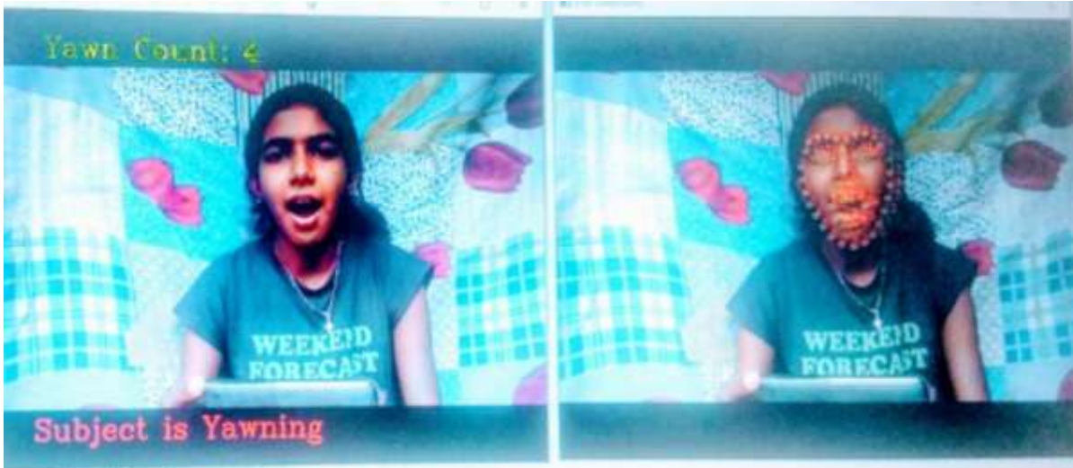
Fig-6: Left: System output while the subject is yawning Right: Detected facial landmarks
