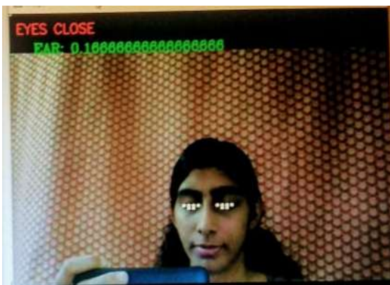
Fig 6 : System output when eyes are closed
