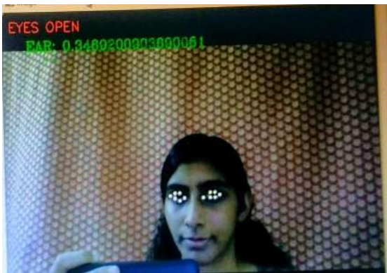
Fig-5: System output when eye is opened
