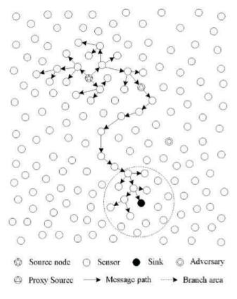
Fig -1: Demonstrates the basic idea of the anonymous routing scheme.
