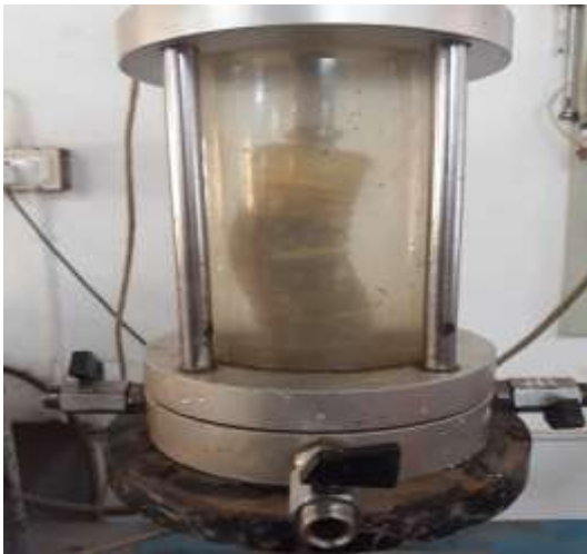
Fig- 5: Bulging of soil sample in tri axial test
