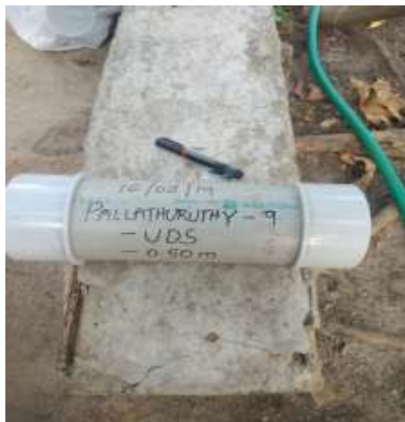
Fig- 1: Collected soil using PVC pipe
