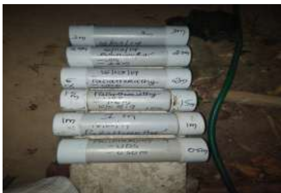
Fig- 2: Collected soil samples from six different depths
