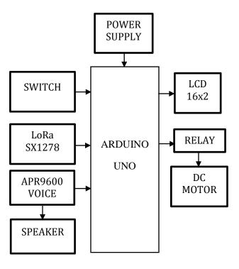
**Fig-3**: Block diagram of the transmitter section.
