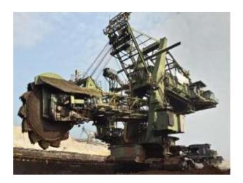
Fig-1: BUCKET WHEEL EXCAVATOR
