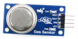
Fig - 3: MQ2 sensor
