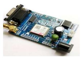
Fig -8: GSM Module
