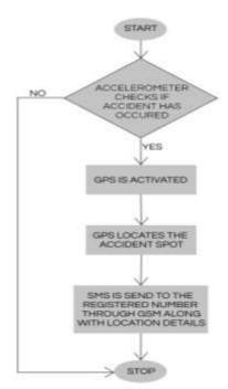
Fig -11: Accident Detection
