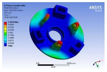
Fig-4: Total Deformation
