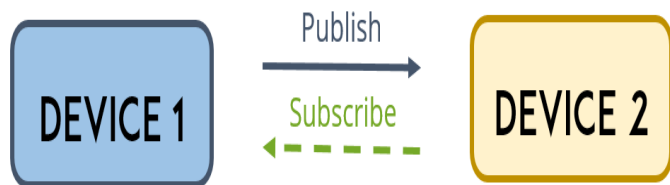
Fig 4: MQTT publishing and subscribe to different devices
