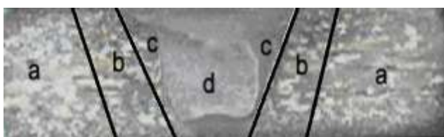
Fig 3- Different regions in FSP (a) Unaffected base metal (BM) (b) Heat affected zone (HAZ) (c) Thermo-mechanically affected zone (TMAZ) and (d) Stir zone (SZ)
