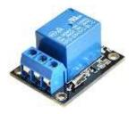
Fig 4.5 Relay Module
