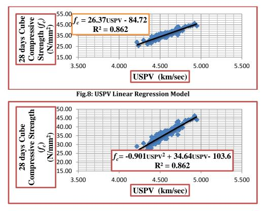
Fig.9: USPV Quadratic Parabolic Regression Model
