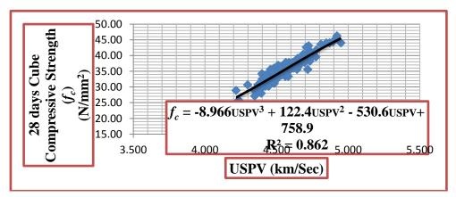
Fig. 10: USPV Cubic Parabolic Regression Model
