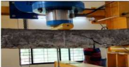
Fig-3: cracks obtained after testing
