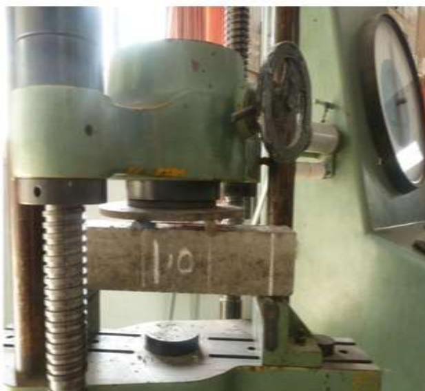
Figure -3: Flexural Strength of Concrete
