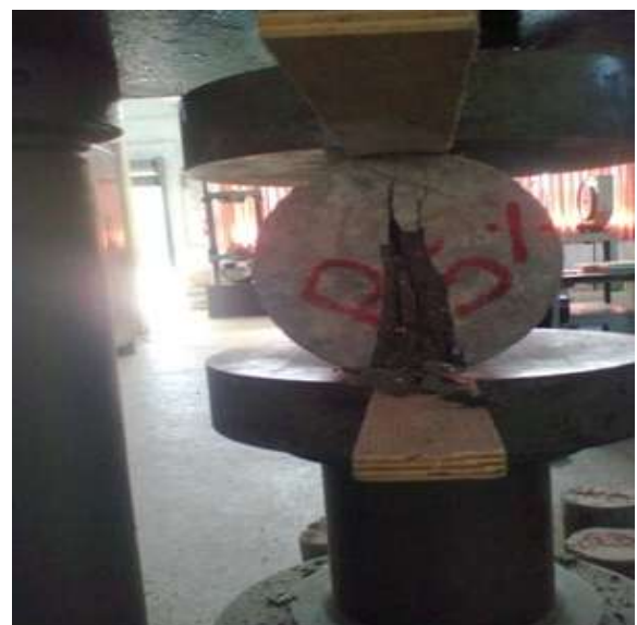
Figure -2: Split Tensile Strength Test
