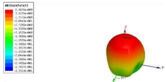
Fig.7 Gain of the E-shape antenna
