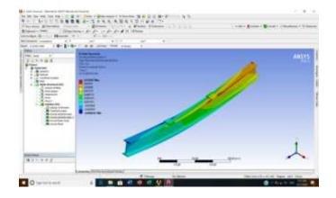
Figure 7. Typical Lateral deflection of FEM Specimen
