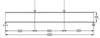
Figure 1. Typical Loading Arrangement of the beam
