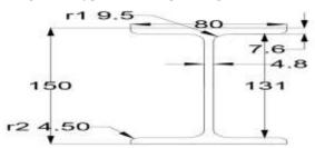
Figure 2. Typical Cross-Sections of the beam
