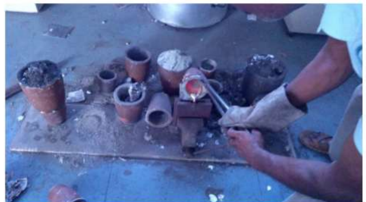
Fig. 4.4 Pouring of molten metal to solidified the alloy
