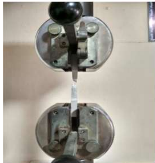
Fig. 6.4 Tensile specimen after breaking
