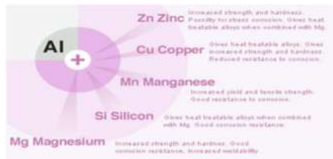
Fig. 2.1 Common alloying elements and their effects in aluminium
