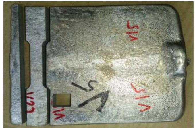
Fig. 5.2 Wire EDM cutting machined sample
