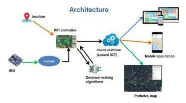
2. Based on the analysis of those algorithm if a pothole is detected by Arduino. It pings Raspberry Pi by sending a low to high pulse at a GPIO of Raspberry Pi.
