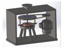
Fig -2: CAD Assembly model of Mechanized quern
