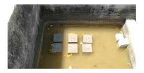
Fig -7: Curing of Cubes
