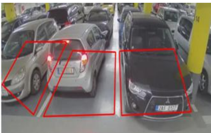
Fig -9: Occupied indoor parking outlined as red by the program (video retrieved from: [7])
