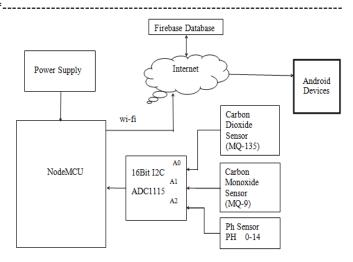
Fig 1.1: Block Diagram of Pollution Monitoring System
