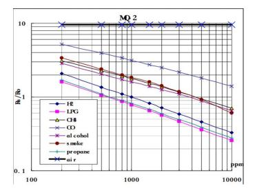
Fig 3.4.1: Logarithmic graph of MQ-2 sensor
