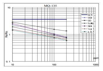
Fig 3.5.1: Logarithmic graph of MQ-135 sensor
