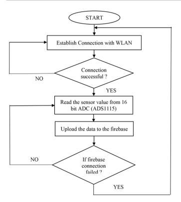
Fig 3.1: flow chart of Arduino program
