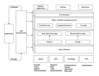
Fig -2: Data Lake Architecture for an Enterprise
