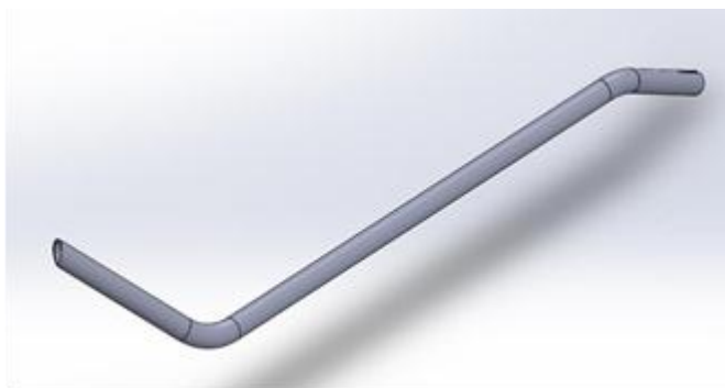
Fig-3: Main Frame Pipe Bend
