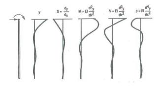
Figure 5: Response of a laterally loaded pile according to Heteyeni
