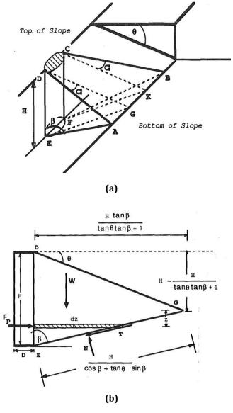
**Figure 8:** Assumed failure wedge with plane failure surface (a) and assumed wedge in equilibrium (b) of Gabr and Borden
