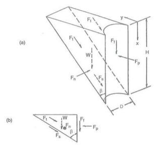
Figure 6: Assumed passive wedge-type failure for clay by Reese et al. [6]
