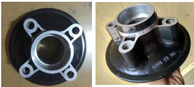
Fig.1: Top view and side view of coupling 4-rubber component
