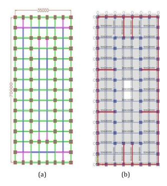
Fig -2: Plan-2 (a) Column and beam layout (b) Outriggerand belt wall layout
