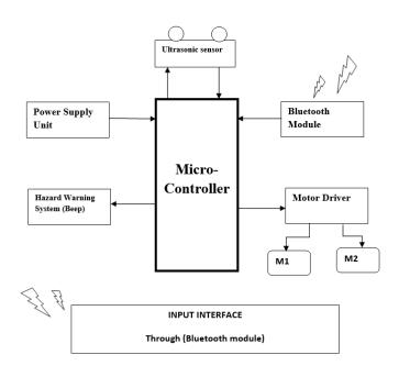
**Fig 1.1** Vehicle Collision Avoidance System Architecture diagram
