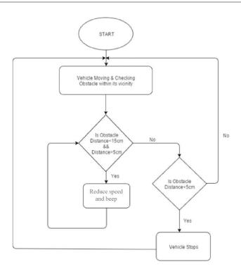
Fig 1.2 Vehicle Collision Avoidance System data flow diagram
