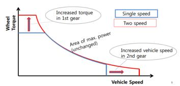
Fig -4: Torque Vs Speed of Two Speed Transmission in EV
