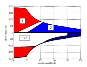
Fig -5: Efficiency at different speed of two speed gearbox in EV
