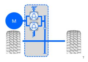
Fig -2: Two speed transmission in EV
