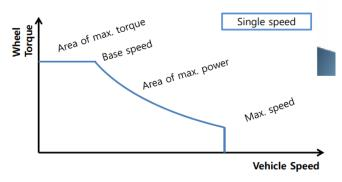
Fig -3: Torque Vs Speed of Single Speed Transmission in EV
