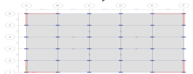
Figure 4.9- Plan of (G+15) storied building with infill wall and shear wall/steel bracing in open ground storey.
