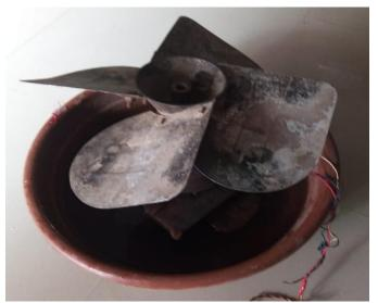
Fig.-2: Bottom fan orientation with water reservoir
