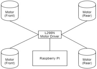
Fig -5: Motor driver connection with the motors
