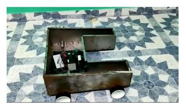
Fig -11: The bot, with top lid open(with components installed)
