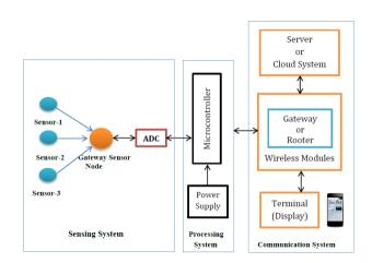
Fig- 3: Typical Architecture of Sensor Node
