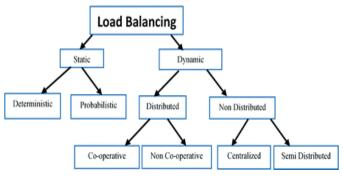
Fig-2: Load balancer types
