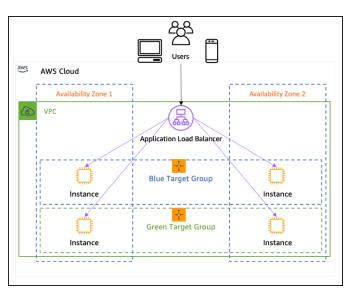
Fig -4: Application load balancing
