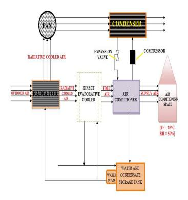
Fig-1: Air conditioner coupled with indirect direct evaporative cooling system
