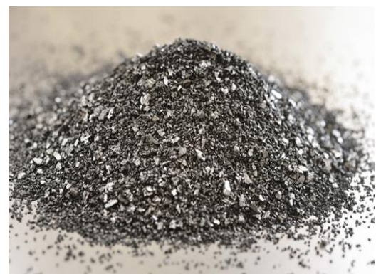
Fig.3 Granular Activated Carbon to be used as an adsorbent.
