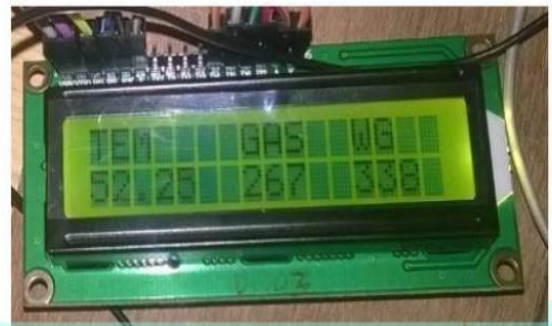
Fig 3.1 LCD showing output of temp, gas level and weight
