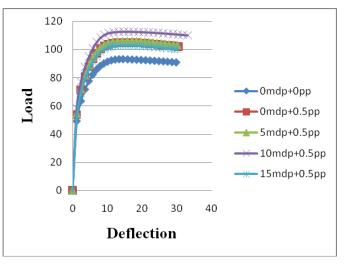
Fig-4: Load-deflection graph of RCC beam
