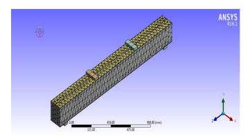
Fig-6: Meshed Partially encased beam
