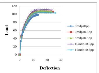
Fig-12: Load-deflection graph of Fully encased beam
