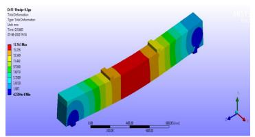
Fig-11: Deflection of Fully encased beam The values obtained after analysis is shown in table 3.
