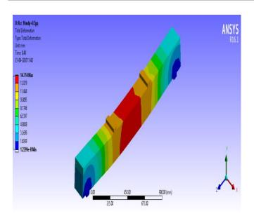
Fig-3: Deflection of RCC beam
