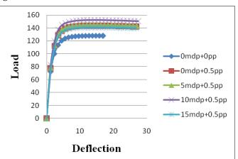
Fig-8: Load-deflection graph of Partially encased beam
