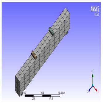
Fig-2: Meshed RCC beam
