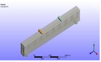
Fig-9: Model of Fully encased beam
