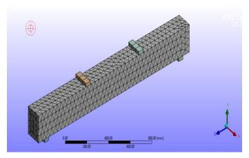
Fig-10: Meshed Partially encased beam
