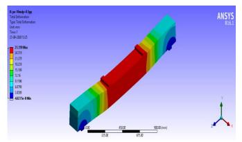
**Fig-7:** Deflection of Partially encased beam The values obtained after analysis is shown in table 2.
