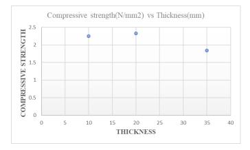
From the above performed experiments, it is observed concrete block with **EPS** Sheet 150mmX70mmX35mm have less compressive strength (1.5 N/mm2) as compared. Hence, as the sheet size increases there is decrease in density of cement as well as decrease in amount of aggregates used thus leading to decrease in compressive strength. Whereas, **EPS** concrete block with sheet 130mmX70mmX20mm have more compressive strength (2.326 N/mm2).
