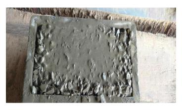
Casting of Blocks (190mmX90mmX55mm)
