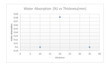
C. Testing on EPS Blocks having dimensions-1.110mmX70mmX35mm 2.110mmX70mmX20mm 3.110mmX70mmX10mm
