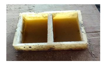
Dry mix containing cement, sand, coarse aggregate was prepared and mixed for about 2 minutes. It was then transferred into molds kept on vibrator machine for minute.
