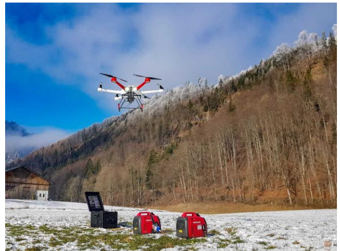
Fig -1: Tethered Mothership Drone (MD) with ground-base (black) and two mobile power supply units (red)
