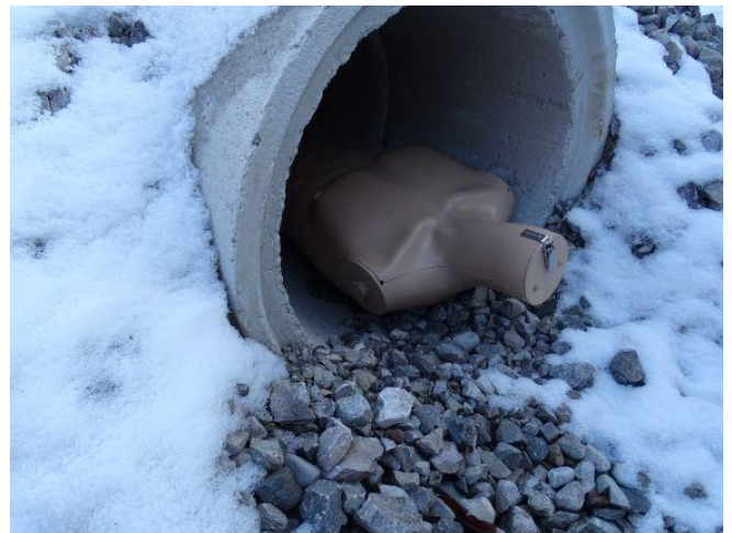
Fig - 10: Test dummy (with breathing simulator inside chest), positioned in concrete tube underneath 12 t of gravel, for ground penetrating radar measurement (radargram)
