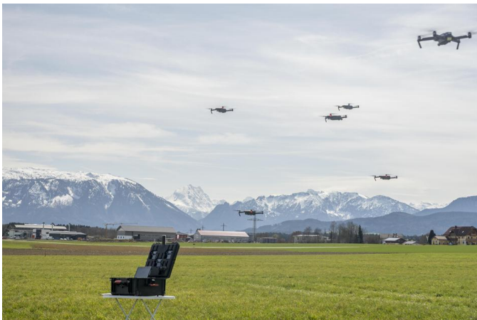
Fig - 4: Five drones used for modelling swarm (MSD), with 6 th drone filming swarm in operation
