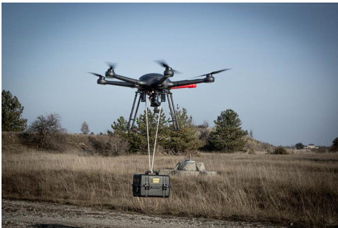
Fig -2: Ground Penetrating Radar Drone (GPRD) transporting radar sensor
