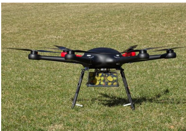
Fig -3: Transport Drone (TD) transporting SMURFs in special container with remotely controlled release
