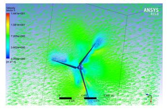
Fig -8: CFD result for 7 m/s wind speed
