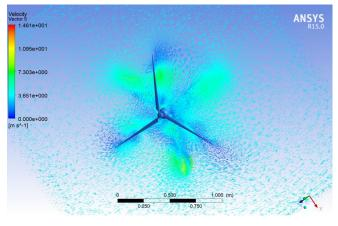
Fig -6: CFD result for 3 m/s wind speed
