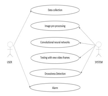
FIG - 2: Use Case diagram of Drowsi Care System.
